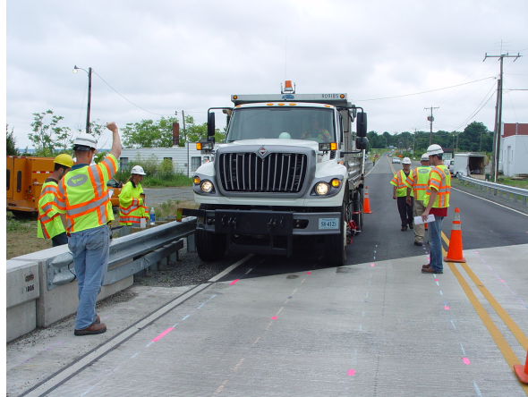
Figure 13 – Static Load Testing with Truck Guided Along Wheel Path A
